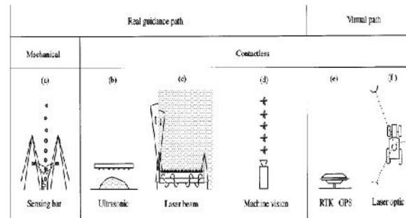
Fig. 3: Automatic steering systems of farm machines: (a) mechanical sensing bars; (b) ultrasonic sensors; (c) laser beam reaction; (d) machine vision; (e) real-time kinematic global positioning system and (f) laser optic navigation
