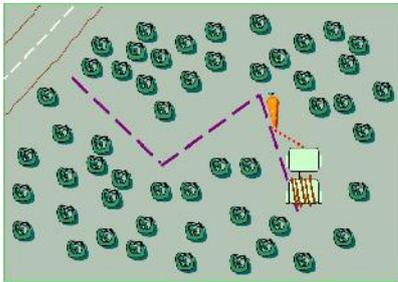
**Fig.4:** AGV following a path by waypoints. Path tracking by "following the carrot", a method causing the AGV to take shortcuts in sharp turns
