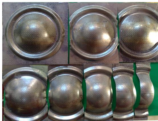
**Fig. 4** Deep drawn samples of painted galvanized steel sheet
