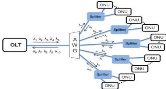
Figure 1 TDM/WDM PON architectures [3]
