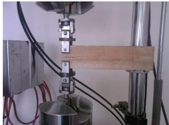
Figure 3 Notched DCB specimen under tensile test
