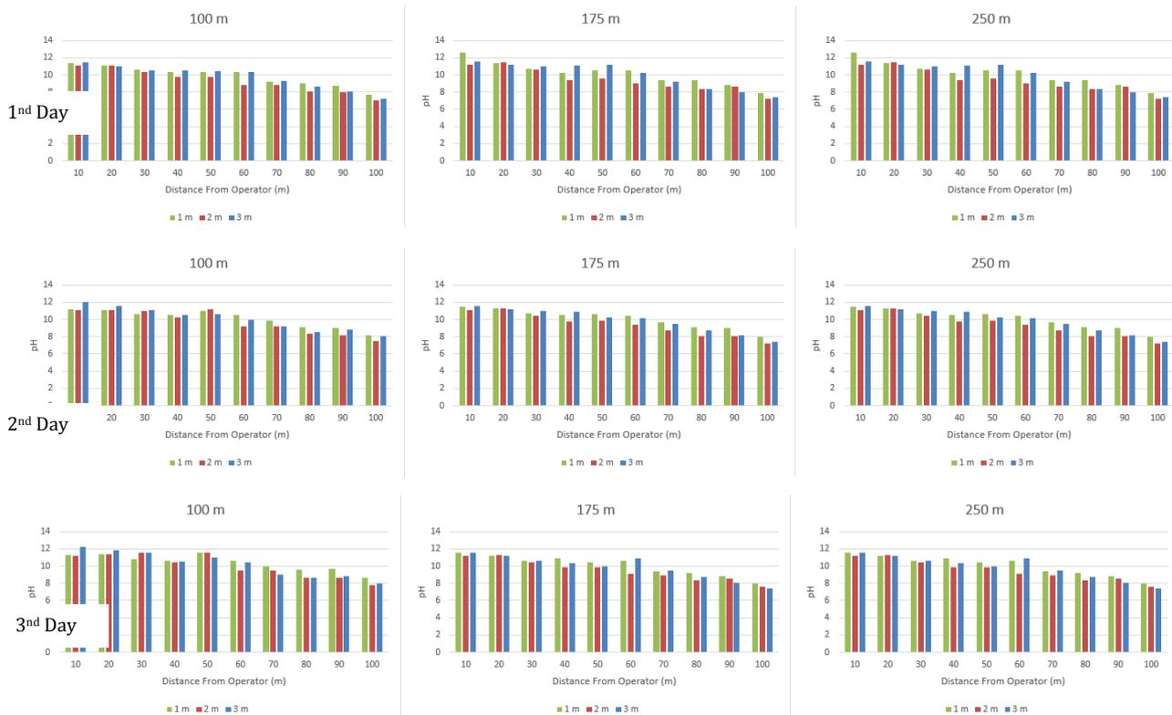
Figure 3 pH variation in different distances from the tunnel opening
